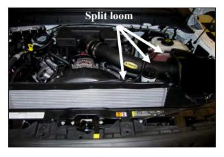
**10.** Slide the 20" section of Split Loom over the Coolant line to protect it from chaffing on the intake tube.
