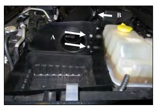
**8. A.)** Mount the Intake Tube to the Rear Panel using the two 1/4-20 Button Head Bolts and 1/4" Flat washers.
