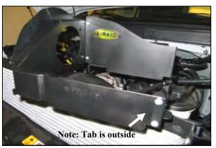
4. Assemble the two Quick Fit panels as shown using four 6-32 screws, flat washers, and kep nuts. Apply the Airaid Foil Decal onto the Panel as shown.
