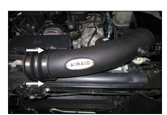
7. Install the Hump Hose, and the clamps onto the Intake Tube. Slide the hump hose and clamps down the tube as far as they will go and leave the clamps loose for now. Apply the Airaid Bubble Decal inside the Airbox as shown.
