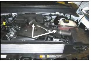
1. Disconnect the negative battery cable! Loosen the two intake clamps, unclip the coolant line, and remove the Factory intake tube.
