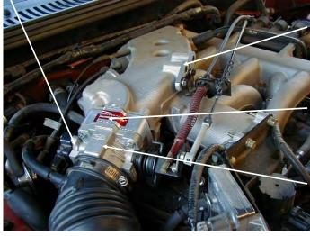
**Ref. "C"-** (2) 6mm Flat Head Screws (1) Linkage Bracket
