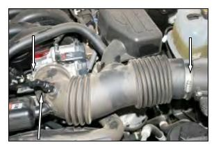
**4.** Re-install the factory intake tube onto the throttle body and the airbox lid, and tighten the hose clamps. Re-connect the breather hose to the factory intake tube.
