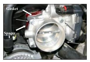
3. Insert the four 6mm x 75mm bolts (#3) with washers (#4) thru the throttle body, one gasket (#2), and thru the Airaid Spacer (#1), and into the intake manifold. Tighten all four throttle body bolts evenly, to the manufacturer's specifications. **Do Not Over Tighten** The Bolts!
