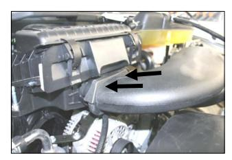
**7.** Install the Airaid Modular Intake Tube (#2) into the factory airbox. It will "snap" into place.
