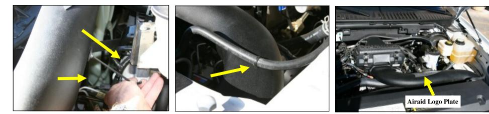
**7.** Install the 1/4"x 20 Allen bolt and washer thru the bracket and into the MIT . Make your final adjustments and tighten the Allen bolt, and the nut on the power steering bracket. The MIT should not make contact with the radiator support or inner fender.
