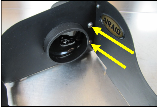
10. Mount the Sensor Tube onto the Panel Assembly and secure using the two 1/4-20 Button Head Screws and 1/4" Flat Washers.
