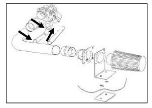
15. 4.6L engines continued: Connect the Airaid Intake Tube nipple to the *IABV* inlet tube using the  $3/4 \ge 1/2$ " L-hose (#7), and two #22 speed clamps (#17).
