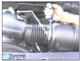
**2.** Loosen the hose clamps at the throttle body, and air filter housing outlet.
