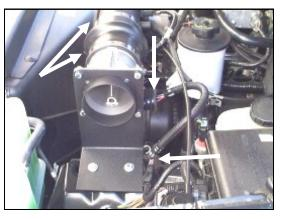
**9.** Reconnect the **MAF** sensor wiring harness to the sensor, and to the main engine wiring harness. Install the urethane hump hose (#4) onto the **MAF** sensor, with two #60 hose clamps (#13). Tighten only the clamp on the sensor.
