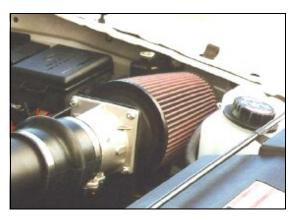
16. Install the Airaid Premium Filter (#1) onto the MAF bracket, and tighten the clamp. Reinstall the beauty cover using the three factory bolts.
