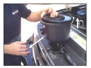
**5.** The factory airbox assembly is held in place by rubber grommets (it is a "pull to release fit."). Remove the assembly and grommets from the engine compartment. Unlatch the airbox and separate the
