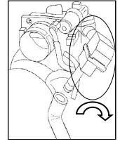
14. <u>4.6L engines</u>: Rotate the *IABV* inlet tube 90 degrees to provide clearance for the 3/4 x 12" Lhose (#7).
