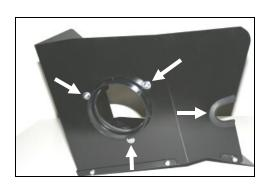
**10.** Install the air filter adapter (#2) into the **CAD** using three  $\frac{1}{4}$  - 20 x 1/2" button head bolts (#14) and  $\frac{1}{4}$ " flat washers (#15). Next, install the 4" rubber trim (#23), as shown.
