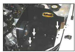
12. Install the CAD into the vehicle with one 6mm bolt (#16) and 1/4" flat washer (#15) through the panel, through the coolant reservoir mount and into the speed nut below it. Using two 6mm bolts (#16) two 1/4" flat washers (#15), two 1/4" lock washers (#17), and two M6 hex nuts (#18), insert the two bolts thru the CAD, thru the grommets, and thru the long/narrow bracket (#19). Use the line drawing above for reference.
