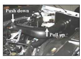
15. While gently lifting on the tube next to the radiator, and pushing down on the tube over the throttle body, tighten the two button head bolts on top of the mounting brackets. This will help make sure the Airaid Intake Tube is sealing on the throttle body.
