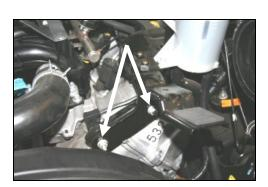
**17.** Factory tolerances may require adjusting the factory bracket to align the tube and hump hose with the filter adapter. Therefore, it may be necessary to loosen the two mounting nuts with a 13mm deep socket, and adjust it.
