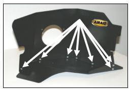
9. Assemble the two Cool Air Dam (CAD) panels (#3, #4) using seven 6-32 x 5/16° screws (#11), #6 flat washers (#12), and 6-32 keps nuts (#13). Apply the Airaid Decal as shown.
