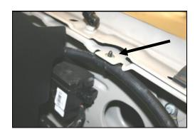
**18.** Slip the black plastic hose mount (#26) over the radiator overflow hose. Next, place one ½" flat washer (#15) over the hole on the inner drivers side fender. Slide the hose mount prongs thru the fender and thru the washer.
