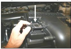
**4.** Using the provided T-20 Security Bit, remove the two screws, and remove the **MAF** sensor from the factory intake tube. Save the sensor for re-installation in the next step.
