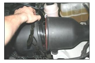
1. Disconnect the negative battery cable. Unclip the factory airbox from the factory Mass Air Flow (MAF) sensor housing.
