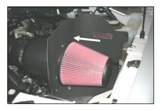
**13.** Mount the Airaid Premium Filter (#1) onto the filter adapter and tighten the clamp.
