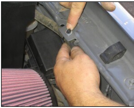
13. Mount the factory coolant hose to the inner fender using the supplied black plastic hose mount and washer as shown above.
