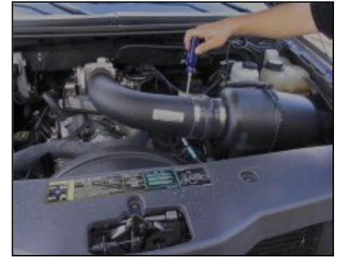
20. Tighten hose clamps on both ends of the Modular Intake Tube.
