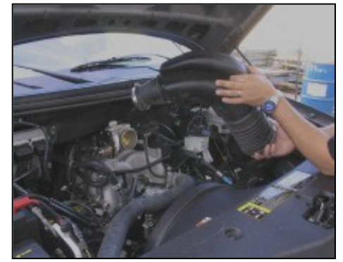
16. Remove the factory intake tube assembly from engine.
