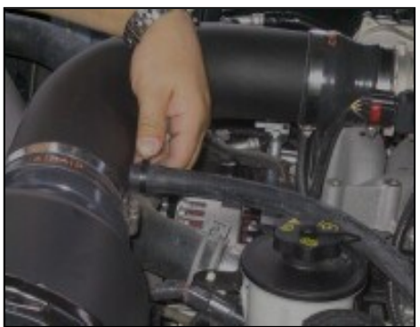
21. Install the supplied rubber hose on the Modular Intake Tube. Connect the other end of the hose to the valve cover. Secure both ends of the hose with the supplied speed clamps.
