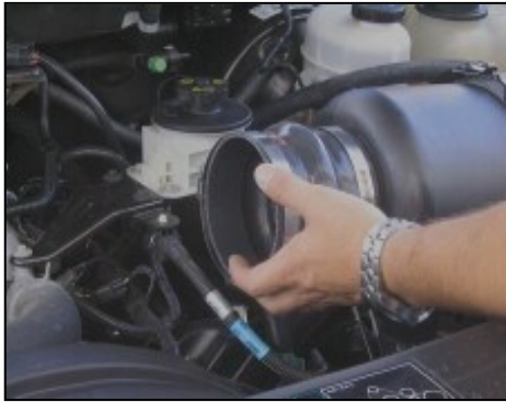
17. Install the supplied urethane hump hose and two #80 hose clamps on factory air filter assembly. Leave hose clamps loose until final assembly.
