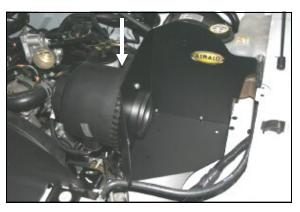
11. Install the CAD assembly into the vehicle. First, align the filter adapter with the factory MAF sensor housing, then, secure it with the factory clamp.
