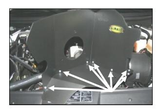
**5.** Assemble the Airaid Cool Air Dam (CAD) panels (#2, #3) using seven 6-32 x 5/16" screws (#9), #6 flat washers (#10), and 6-32 keps nuts (#11). Apply the Airaid Foil Decal onto the Panel as shown.
