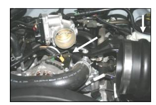
**14.** Using a 10mm socket, remove one factory bolt from under the throttle body. Using a 5/32" allen wrench, install the M6x1x20 button head bolt (#26) in its place. Install the urethane hump hose (#6) and two #80 hose clamps (#25) onto the factory MAF sensor housing. (Leave the clamps loose for now).
