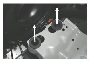
**9.** Remove the two factory grommets from the factory airbox mounting plate.
