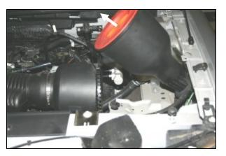
**2.** Remove the factory air filter and airbox from the vehicle. Pull straight up on the airbox, to release it from the grommets, and then remove the airbox inlet from the drivers side fender.
