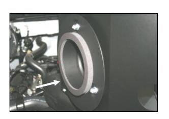
7. Install the gasket (#16) onto the filter adapter.
