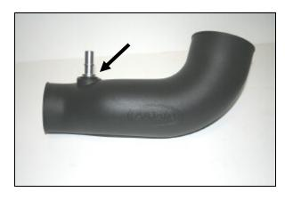
**8.** Install the rubber grommet (#22), and aluminum fitting (#21) into the Airaid Intake Tube (#4).
