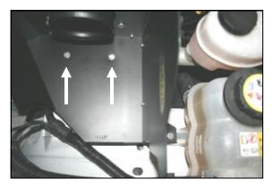
13. Insert two  $\frac{1}{4}$  - 20 x 7/8" bolts (#12) and  $\frac{1}{4}$ " flat washers (#13) through the holes in the CAD and thru the grommets. On the underside of the factory airbox mounting plate, align the long/narrow bracket (#19), two 1/4" flat washers (#13), and two  $\frac{1}{4}$  - 20 locknuts (#15) with the  $\frac{1}{4}$ -20 x 7/8" bolts. Tighten the assembly securely.
