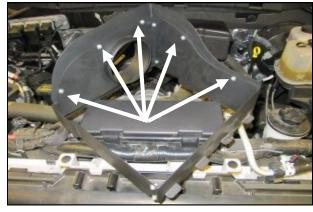
**5. For F-150 models only:** Fasten the Extension panel (#5) to the outside of the panel assembly using the remaining 6-32 screws, flat washers, and kep nuts.
