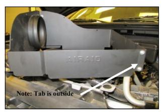
**4.** Assemble the two Quick Fit panels (#3 & #4) as shown using four 6-32 screws (#9) flat washers (#11) and kep nuts (#10).
