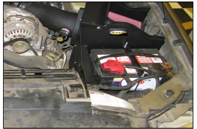
18. Double check your work! Make sure there is no foreign material in the intake path. Make sure all clamps, hoses, bolts, and screws are tight. Double check the hood clearance. Reconnect the battery cables.
