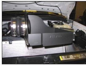
**5. A.)** Install the Silicone Hump Hose (#6) and two #64 Hose Clamps(#14) onto the Quick Fit assembly. Leave the clamps loose for now.
