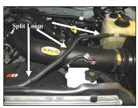
9. A.) Insert the Airaid Intake Tube into the couplers as shown. Check for alignment, and tighten all clamps.
