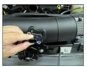
**8.** Transfer the **MAF** sensor into the Airaid Intake Tube (#2) and secure using two 8-32 x 3/8" button head screws (#12). **Do Not Use The Factory Torx Head Screws!**
