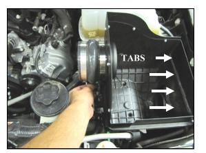
**5. A.**) Install the Silicone Hump Hose (#7) and two #64 Hose Clamps(#14) onto the Quick Fit assembly. Leave
