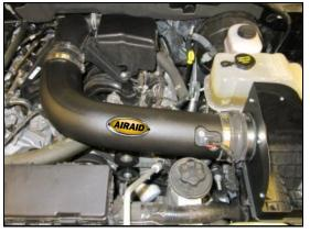
8. A.) Insert the Airaid Intake Tube into the couplers as shown. Check for alignment, and tighten all clamps.B.) Re connect the Mass Air Flow Sensor. Apply the Airaid Bubble Decal onto the Intake Tube as shown.
