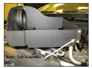
**4.** Assemble the two Quick Fit panels (#3 & #4) as shown using four 6-32 screws (#9) flat washers (#11)
