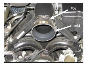
**6.** Install the Silicone Coupler (#6), one #64 Hose Clamp(#14), and the #52 Hose clamp (#13) onto the
