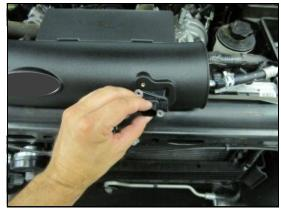
7. Transfer the MAF sensor into the Airaid Intake Tube (#2) and secure using two 8-32 x 3/8" button head screws (#11). <u>Do Not Use The Factory Torx</u> <u>Head Screws !</u>
