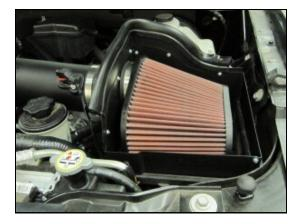
**9.** Install the Airaid Premium Filter (#1) to the mounting flange inside the quick fit assembly. Complete the installation by attaching the Weather Strip (#5) to the top of the panels as shown.
