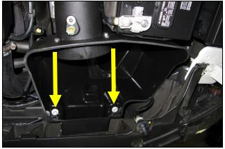
11. Place the Airaid Intake assembly in the original loca- 12. Slide the coupler and clamps onto 90 deg. Elbow pipe tion of the Factory Air box and secure using the factory and tighten the clamps. hardware from step 4. Slide the coupler and clamps onto 90 deg. Elbow pipe and tighten the clamps.
