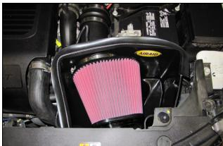
14. Plug the Harness Extension into the factory wire har- 15. Install the Airaid Premium filter onto the Filter onto the top of the Air box as shown, with the contour rolling away from the filter.
