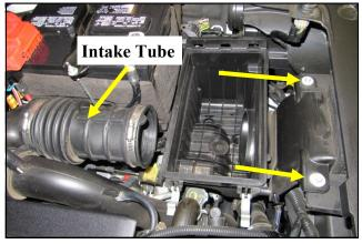
**4.** Using an 8mm socket, remove the two factory air box **5.** Remove the factory air box assembly from the vehicle. bolts and set aside. The will be reused in step 11. Loosen Be sure to retain the two air box mounting grommets. the second intake tube clamp and remove it from the ve-
