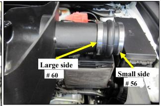
**8.** Install the Hump Hose, large side first onto the Intake tube. Loosely install the #56 Hose Clamp on the small side of the Hump Hose, and the #60 Hose Clamp on the Large side. Slide the Hump Hose and Clamps downward onto the tube, as far as it will go, creating a compact assembly as shown.
