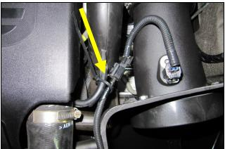
ness and secure it using the supplied Zip Tie. Trim the Adapter and tighten the clamp. Install the weather strip excess length
