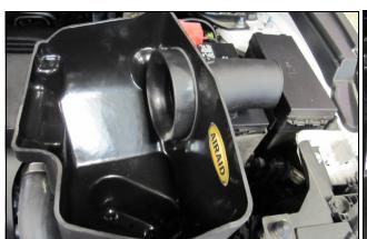
7. Install the Filter Adapter to the inside of the Cool Air Box, using the three 1/4"-20 hex head bolts and 1/4" flat washers. Apply the Airaid Bubble Decal inside the Airbox as shown.
