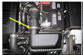
1. <u>Disconnect the negative battery cable.</u> Loosen the clamp on the air box side of the intake tube.
