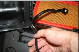
**3.** Using a pair of needle nose pillars, carefully compress the fins of the wiring harness anchor and pull it out of the air box lid.
