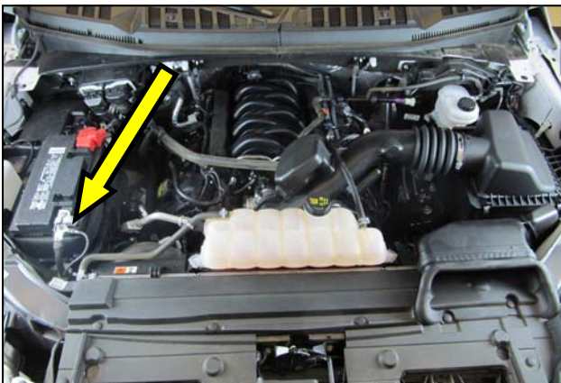
1. Disconnect the negative battery terminal.
