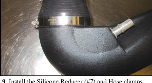
**9.** Install the Silicone Reducer (#7) and Hose clamps onto the Airaid Intake Tube (#2). Place the #56 clamp (#15) on the Throttle body side of the reducer, and the #64 clamp (#17) on to the tube side.
