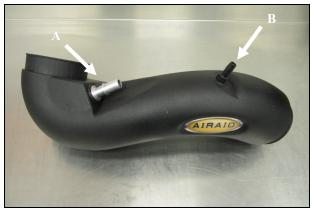
**8. A.)** Insert the 5/8" Grommet (#18) into the Intake tube as shown. Complete the tube assembly by inserting the 5/8 PCV Fitting (#16) into the Grommet. **B.)** Install the 3/8 "Hose Fitting (#20) into the threaded holt in the Intake Tube. Complete the Tube assem-
