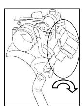
**15.** 4.6L engines: The idle air bypass line goes directly to the throttle body. Rotate the resonator box 90 degrees to provide clearance for the 3/4 x 12" L-hose (#7). Install the 3/4"x12" L-hose (#10) onto the Airaid Intake tube and the resonator box and secure it using the two #22 speed clamps (#23).
