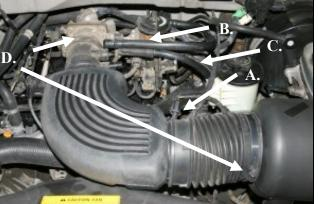
2. A) Very carefully, using a pulling circular motion, remove the air intake temperature sensor from the air intake tube. **B)** Disconnect the upper, idle air bypass hose. C) Disconnect the crankcase breather at the intake tube and the valve cover, and remove it from the vehicle. **D**) Loosen two hose clamps and remove the air intake tube from the vehicle.
