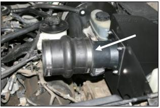
11. Install the hump hose (#7) onto the MAF sensor housing as shown using two #60 hose clamps (#21). Tighten only the clamp on the MAF sensor housing at this time.
