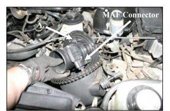
4. Unlatch the clamp on the canister to separate the two halves. Once separated, remove the factory air filter. A) Next, slide the large round plastic Mass Air Flow (MAF) sensor adapter plate from the canister. To do this, slide the wires thru the rubber grommet to gain access to the MAF sensor wiring connector. Now disconnect the MAF sensor wiring harness, and remove the MAF sensor housing and adapter plate. Remove the remaining half of the canister from the vehicle.
