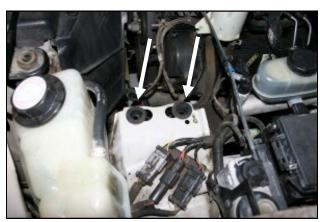
9. Remove the two grommets that held the air filter canister in place. They will not be reused.
