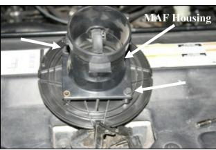
to the adapter. Separate the adapter plate from the MAF sensor housing and save the sensor and housing for reinstallation in step #7.
