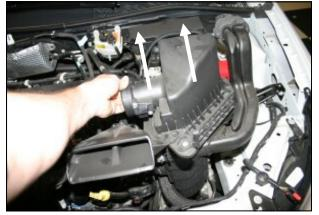
**4.** Pull straight up, and remove the airbox assembly from the vehicle. It is only held in by one grommet at this point.
