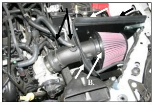
16. A.) Reinstall the small breather hose into the grommet on the top of the intake tube. Reconnect the large breather connector to the factory elbow. B.) Next mount the Airaid Premium Filter (#1) onto the intake tube as shown and tighten the clamp. C.) Install the weatherstrip (#6) onto the top of the CAD panels as shown. Start at the front of the vehicle and work your way towards the fender.
