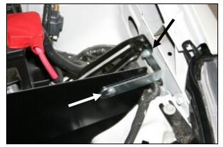
**15.** Install the side bracket (#17) onto the **CAD** as shown using the factory bolt removed in step #6, and one 1/4"-20x5/16 hex bolt (#13), two 1/4" flat washers (#12), and one lock nut (#14).
