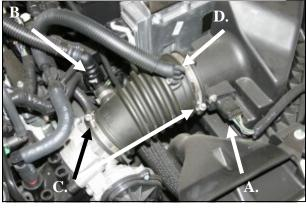
2. A.) Pull the red tab on the bottom, and then squeeze the Mass Air Flow sensor wiring connector and disconnect it from the sensor. B.) Push the tab, and disconnect the breather hose from the plastic elbow. C.) Loosen the two factory clamps on the flexible intake tube. D.) Remove the Oetiker clamp, and then carefully remove the small plastic elbow from the flexible intake tube leaving the breather hose connected to the elbow.
