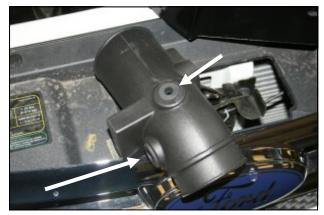
**8.** Install the small grommet (#20) into the hole on the top of the Airaid intake tube (#2). Now install the large grommet (#21) into the hole on the side of the tube.
