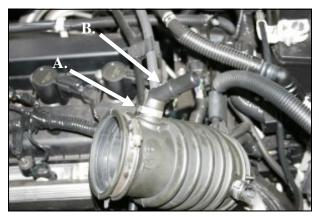
**3.** Remove the factory flexible intake tube from the vehicle. Remove the Oeticker clamp, and then remove the large plastic elbow from the flexible intake tube. It will be reused in step #12.
