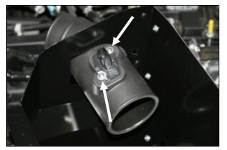
**10.** Insert the Airaid intake tube thru the **CAD** panel and then reinstall the Mass Air Flow sensor from step #5 using the two supplied 8-32x3/8" button head screws (#15). **Do Not Use The Factory Screws!**
