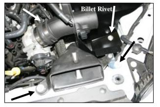
14. Install the CAD into the vehicle making sure to slip the intake tube into the hump hose as you lower the assembly into place. After you have the intake tube correctly located into the hump hose, insert the billet rivet (#19) thru the **CAD** and into the factory grommet in the inner fender well. Tighten the hose clamp on the hump hose and then reinstall the two factory bolts removed in step #1 that secure the scoop to the radiator support. Reconnect the Mass Air Flow sensor!
