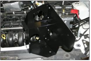
**9.** Auto Transmission vehicle only: Assemble the two Cool Air Dam panels (#3 & #4) using 7 screws (#8), washers (#9), and nuts (#10) as shown. Make sure that the bent flanges where the panels screw together, are on the outside of the box. Note: Use panel #3 with tag marked "AUTO".
