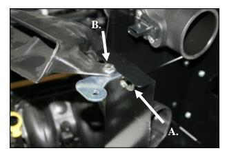
**13. A.**) Install the front bracket (#18) onto the front of the **CAD** as shown using one 1/4"-20x5/8" hex bolt (#13), two 1/4" flat washers (#12), and one lock nut (#14). **B.**) Next mount the factory scoop to the bracket as shown using one 1/4"-20x5/8" hex bolt (#13), two 1/4" flat washers (#12), and one lock nut
