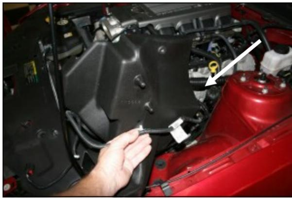
5. Turn the CAD so that the bottom faces the left fender as shown. Now reinstall the wiring loom anchors into their respective holes starting at the back of the CAD with the two hole anchor and work your way underneath and towards the front. The last anchor nearest the MAF sensor is not anchored.
