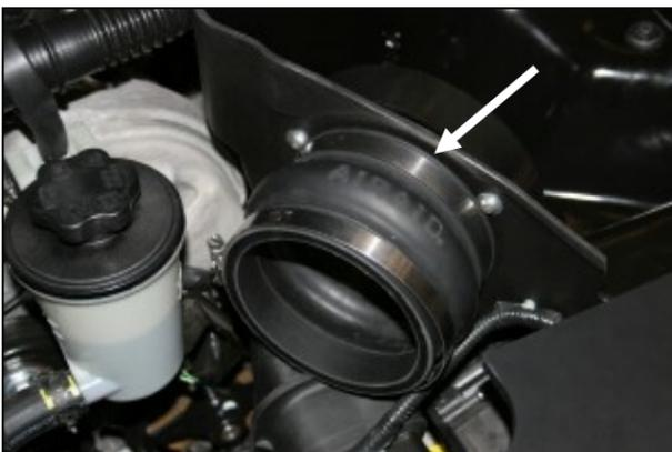
7. Install the provided hump hose (#5) onto the filter adapter using two #72 hose clamps (#17) as shown. Leave the two hose clamps loose for now.
