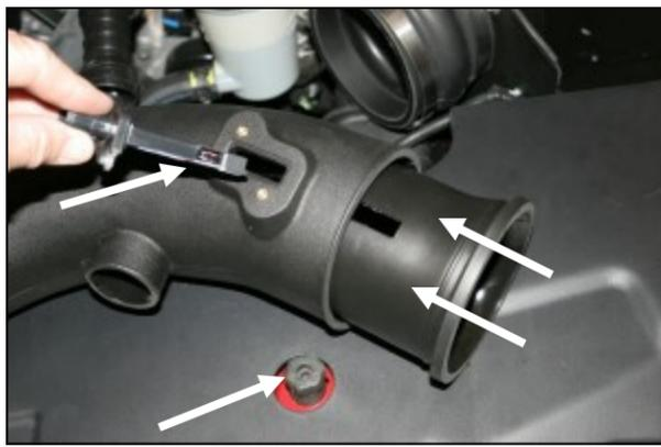
8. Slide the Modular Venturi Tube (#3) into the Airaid intake tube (#2) making sure to align the two slots for the MAF sensor. Next install the MAF sensor into the intake tube using two provided 8-32x3/8" screws (#14).
