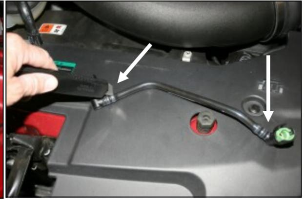
15. **VERY CAREFULLY!** Without cutting thru the connectors, cut the factory breather tube on each end just enough to remove the factory connectors.
