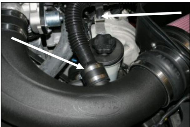
1. Loosen the clamps on the resonator tube coupler and disconnect it from the intake tube. Pull up on the resonator tube to release it from the resonator bracket.
