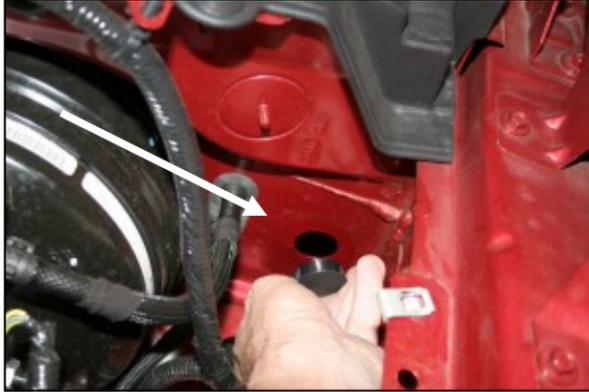
7. Install the optional firewall plug (#20 on the main page) into the hole in the firewall.
