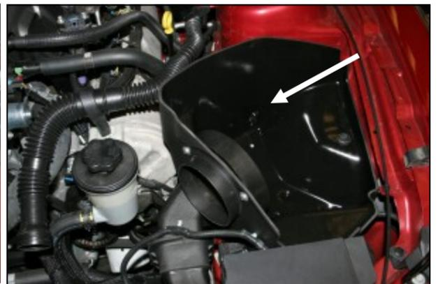
6. Install the CAD into the vehicle making sure that the scoop provision in the CAD aligns with the factory scoop, and the two locating pins on the bottom align with the factory grommets. Next reinstall the factory bolt that was removed in step #2 thru the steel sleeve and grommet and into the inner fender. Make sure that the wiring harness is not pinched under the CAD.
