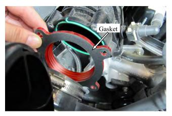
**3.** Pull the throttle body away from the intake manifold and Install the spacer and the supplied gasket. The logo is to be facing the throttle body and in the 12:00 o'clock position. the supplied gasket is to be on throttle body side. Align the bolt holes, and install the supplied bolts and washers. Tighten the bolts to the factory specifications in an "X" pattern. Before starting the engine, manually cycle the throttle plate to make sure there are no obstructions.
