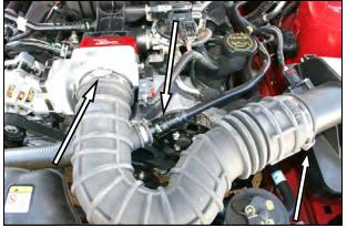
4. Reinstall the intake tube, and tighten the hose clamps.
