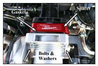
3. Install two bolts (#2), and washers (#3) thru the throttle body, thru the gasket (#4), thru the Airaid Spacer (#1), and into the intake manifold as shown. Use caution to retain the factory o-ring gasket on the plastic intake manifold.
