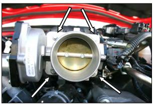
2. Using a 5/16" socket, remove the 4 bolts that hold the throttle body to the intake manifold.
