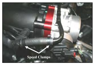
**6.** If you have a three piece breather hose and spring clamps, and replace them with the supplied Breather hose and Speed clamps. Re-torque the throttle body bolts in a X pattern, to Factory spees.
