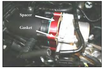
**4.** Position the AIRAID Spacer between the throttle body and the intake manifold with the supplied gasket next to the throttle body as shown. Make sure the "flow" arrow that is printed on the spacer is pointing towards the intake manifold. Insert the provided bolts and washers through the throttle body, gasket, and AIRAID Spacer.
