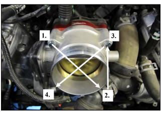
**4.** Insert the provided bolts with washers through the throttle body, gasket, and AIRAID Spacer and tighten them in an "X" Pattern
