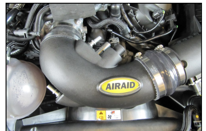
9. Insert the Intake Tube into the Hump Hose and Reducer then tighten all 4 Intake Clamps. Apply the Airaid Bubble Decal onto the Intake Tube as shown.
