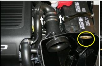
11. A.) Place the CAB in the original location of the Fac- 12. Install the Airaid Premium Filter (#1) onto the Filter tory Air box and secure using the factory hardware from adapter and tighten the clamp. step 4. B.) Slide the coupler and clamps onto 90 deg. Elbow pipe and tighten the clamps. C.) Reconnect the Air Temperature Sensor. Apply the Airaid Decal inside of the Airbox as shown.
