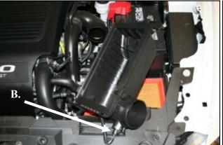
2.A.) Unfasten the factory air box clips and separate the 3. Using a pair of needle nose pillars, carefully compress upper half of the air box from the intake assembly. B.) Disconnect the air temperature sensor.
