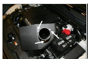
7. Install the Filter Adapter to the inside of the Cool Air 8. A) Install the Hump Hose, large side first (#4) onto Box, CAB (#2) using the three 1/4"-20 hex head bolts (#6) and 1/4" flat washers (#7) as shown.
