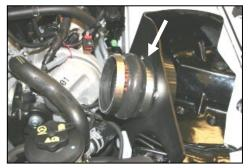
**10.** Install the hump hose (#4) on the filter adapter (#6), with two #72 hose clamps (#12). Tighten <u>only</u> the clamp next to the **CAD**.
