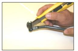
**16.** <u>VERY CAREFULLY !</u> Using a razor blade, cut the plastic tube off both of the factory breather hose ends as shown.
