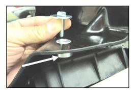
Install the air filter adapter (#5) into the Cool Air Dam (#7) as shown, using 3 button head bolts (#9) and <sup>1</sup>/<sub>4</sub>" flat washers (#10).
