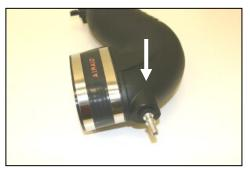
**13.** Install the oval coupler (#3) with two #72 hose clamps (#12). Tighten <u>only</u> the clamp closest to the aluminum fitting. (*Hint: For a clean look, locate the hose clamp tightening screws under the tube)!*
