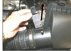
**5.** Using the provided #20 torx bit, remove two screws and the mass air sensor from the factory airbox lid. Note the direction of the sensor for proper re-installation later. (Save the mass air sensor for re-installation in step #13, the factory screws will not be re-used).
