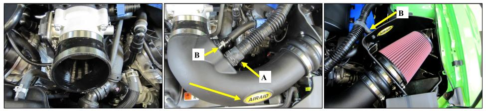
**10.** Install the Silicone Reducer (#6) and Hose clamps onto the throttle body. Place the #56 clamp (#15) on the Throttle body side of the reducer, and the #64 clamp (#14) on to the tube side.
