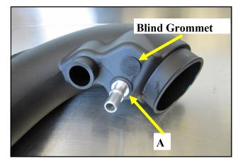
4. Install the Grommets and Fittings into the Airaid intake 5. Using the supplied Torx driver, remove the MAF sentube A) All models will require the use of the 5/8" Fitting sor from the factory airbox and create the Tube assem-(#19) and the 5/8"Grommet (#20). **B)** Automatic trans- bly.
