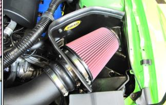
13. Reconnect the Mass Air Flow sensor, which is now 14. Install the Weather Strip onto the Cool Air Box with the contoured edge rolling away from the filter. Start at the front of the vehicle and work your way back
