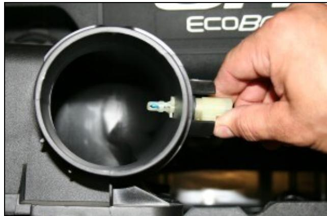
7. Install the Filter Adapter to the inside of the Cool Air Box, CAB (#2) using the three 1/4"-20 hex head bolts (#6) and 1/4" flat washers (#7) as shown.
