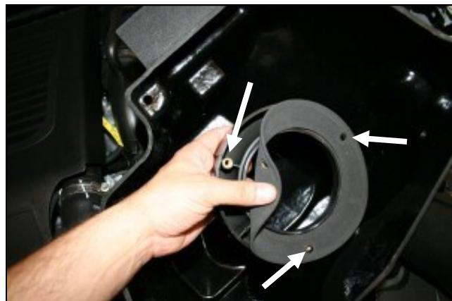
4. A.) Using an 8mm socket, remove the two factory air box bolts and set aside. The will be reused in step 11. B.) Remove the factory air filter element.
