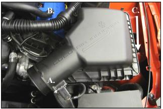
**3. A)** Slide the red tab out of the connector and disconnect the Mass Air Flow sensor. Carefully pry the harness anchor from the air box using a standard screwdriver. **B)** Separate the resonator tube from the stand off attached to the Air box lid. **C)** Using a 10mm socket, remove the bolt securing the air box to the inner fender and remove the air box assembly. This bolt will be reused in step 12.
