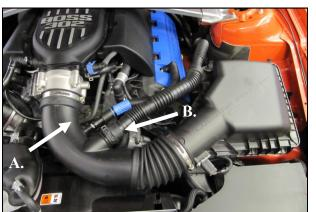
2. A) Loosen the hose clamps on the factory intake tube B) Squeeze the clamp and disconnect the resonator from the air intake tube. C) Carefully depress the hose lock tab and disconnect the crank case breather line. D) Remove the factory intake tube.
