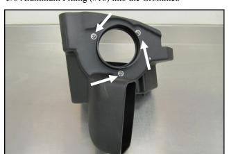
**9.** Install the Filter Adapter (#7) onto the Airaid Cool **A**ir **B**ox (#4) as shown.
