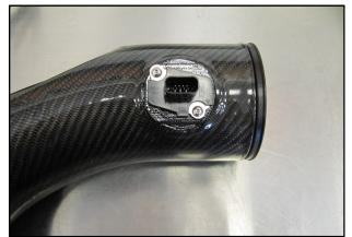
**8.** Install the Mass Air Flow sensor into the intake tube using two provided 8-32x3/8" screws (#11).
