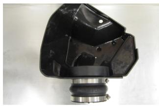
**11.** Install the hump hose (#5) and two #72 hose clamps (#12) onto the filter adapter as shown. Leave the two hose clamps loose for now.
