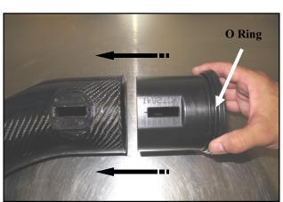
**4.** Unbolt the Intake resonator from the inner fender and disconnect it at the drivers side firewall. Remove the
