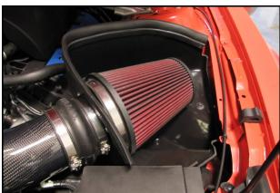
**15.** Install the Airaid Premium Filter (#1) onto the filter adapter and tighten the hose clamp.
