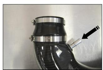
**6. A.)** Install the Silicone Reducer (#6) and Hose clamps onto the Airaid Intake Tube (#2). Place the #56 clamp (#14) on the Throttle body side of the reducer, and the #64 clamp (#13) on to the tube side.
