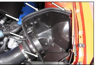
**14.** Install the Weather Strip (#8) onto the Cool Air Box with the contoured edge rolling away from the filter area. Start at the front of the vehicle and work your way back
