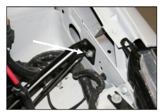
**6.** Remove one bolt that secures the brace to the inner fender. It will be reinstalled in step #15.
