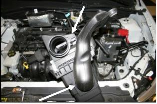
**5.** Remove the scoop from the factory airbox. Next, using the supplied #20 Torx bit, remove the Mass Air Flow sensor from the airbox lid. These parts will be reinstalled in steps #10 & 13.
