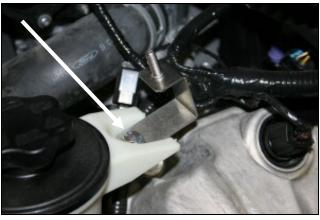
11. Install the bracket assembly from step #10 as shown. 12.A.) Install the oval coupler onto the intake tube using This bracket and 6mm bolt will secure the power steering two #72 hose clamps (#17). Leave the clamps loose for reservoir and replaces the stud removed in step #9.
