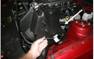
sensor is not anchored.
