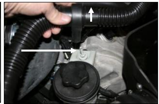
9. Lift up on the intake resonator tube to disengage it from the stud securing the power steering reservoir. Using a deep 10mm socket, remove the stud and save it for a possible optional install. See step #18.
