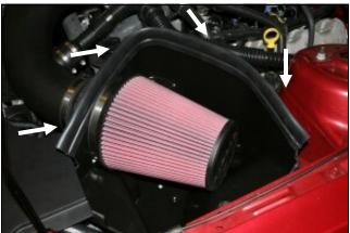
adapter and tighten the hose clamp. Next, install the connectors, cut the factory breather tube on each end just weatherstrip (#11) onto the top of the CAD as shown enough to remove the factory connectors. starting near the radiator and working your way towards the left fender.
