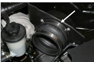
7. Install the provided hump hose (#5) onto the filter 8. Slide the Modular Venturi Tube (#3) into the Airaid adapter using two #72 hose clamps (#17) as shown. Leave the two hose clamps loose for now.
