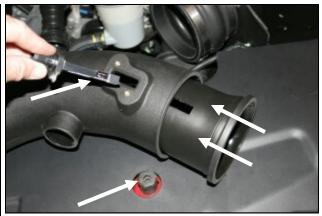
intake tube (#2) making sure to align the two slots for the MAF sensor. Next install the MAF sensor into the intake tube using two provided 8-32x3/8" screws (#14). **Do Not Use The Factory Screws!**
