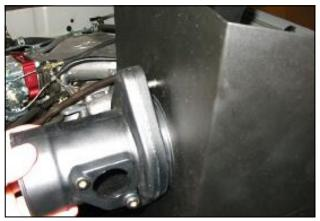
7. Using two supplied 1/4-20 bolts and washers, mount the Airaid filter adapter to the Airaid Cool Air Dam.
