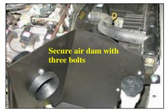
**10.** Position the Airaid intake assembly in place of the original, factory assembly. Using three supplied 8mm bolts and washers, mount the Airaid assembly using the three original/factory mounting points.
