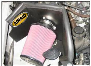
**15.** Mount the Airaid premium air filter inside the Cool Air Dam & press weather strip onto the top of the Cool Air Dam. (*Hint: start at a corner and work towards the ends*) Apply the Airaid Foil Decal onto the Panel as shown.
