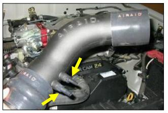
9. Install two supplied 1/4" NPT barbed fittings in Airaid intake tube. (Note: Install 3/8" fitting in the forward hole and the <sup>1</sup>/<sub>4</sub>" fitting in the back hole) Slide hump hose and two #52 hose clamps on large end of intake tube and slide coupler with two #48 hose clamps on small end of tube. (Note: leave all hose clamps loose for final assembly)
