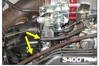
2. Remove factory vacuum lines / hose from the factory air box and intake tube. (*Note: Retain the 3/8*" *vacuum hose*)
