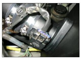
**12.** Reinstall the electrical connector to the Mass Air Sensor.
