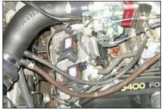
**13.** Connect factory 3/8" vacuum line to nylon fitting on intake tube & connect steel tube on intake manifold to 1/4" fitting on intake tube with 1/4" vacuum line provided.
