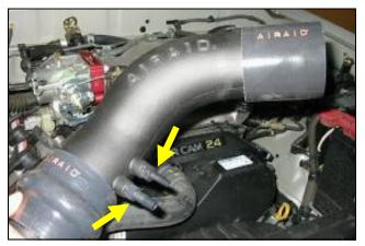
**9.** Install two supplied ¼" NPT barbed fittings in Airaid intake tube. (*Note: Install 3/8*" *fitting in the forward hole and the ¼*" *fitting in the back hole*) Slide hump hose and two #52 hose clamps on large end of intake tube and slide coupler with two #48 hose clamps on small end of tube. (*Note: leave all hose clamps loose for final assembly*)
