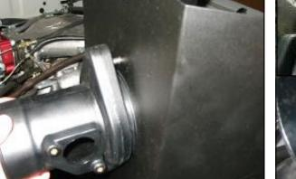
7. Using two supplied <sup>1</sup>/<sub>4</sub>-20 bolts and washers, mount the Airaid filter adapter to the Airaid Cool Air Dam.
