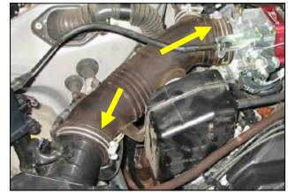
**1.Disconnect The Negative Battery Terminal!** Loosen the two hose clamps on the factory intake tube.
