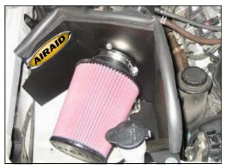
**15.** Mount the Airaid premium air filter inside the Cool Air Dam & press weather strip onto the top of the Cool Air Dam. Apply the Airaid Foil Decal onto the Panel as shown.
