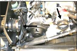
**13.** A) Install the urethane hump hose (#7) onto the MAF adapter (#4). Use the #56 hose clamp (#12) on the MAF adapter end, and the #60 hose clamp (#13) on the intake tube end. B) Install the reducer coupler (#6), small end towards the throttle body with two #52 hose clamps (#11). Leave the clamps loose for now.
