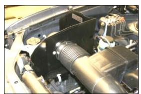
**5.** Slide the **MAF** adapter into the factory tube, and at the same time slip the **CAD** onto the top of the factory airbox base, adjust for fit and relatch the 3 factory clips. Tighten the hose clamp on the factory intake tube. Reinstall the shroud bolt from step #4.
