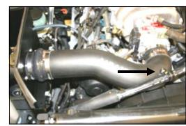
**15.** Install the Airaid **MIT** (#5) into the hump hose first, and then into the coupler. Adjust the MIT snugly against the throttle body and tighten all four clamps. Install the supplied button head bolt (#20), and washer (#21) thru the Adel clamp, and thread into the MIT. (See arrow)
