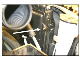
**4.** Remove the fan shroud bolt from the passenger side of the radiator. (Save for reuse).
