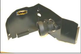
**3.** Assemble the Airaid Cool Air Dam (CAD) panels (#2, #3) using three 6-32 x 5/16" screws (#17), #6 flat washers (#18), and 6-32 keps nuts (#19). Install the MAF adapter (#4) using two 1/4 - 20 button head bolts (#20), and 1/4" flat washers (#21). Apply the Airaid Foil Decal onto the Panel as shown.
