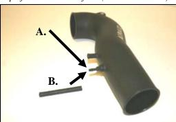
14. A) Install the 1/4"Barb x 1/8"NPT fitting (#14) into the Airaid Modular Intake Tube
