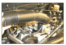
12. Remove the factory intake tube.
