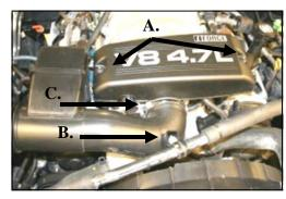
10. A) Using a 10mm socket, remove the two nuts and remove the beauty cover. (Save for reinstallation.) B) Remove the bolt thru the Adel clamp for the air conditioning hose. C) Loosen the hose clamp on the factory intake tube at the throttle body and the airbox if it was tightened in step #5.
