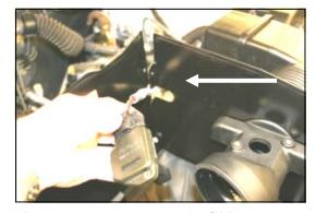
**6.** Remove the top screw on the **CAD**. Spread the panels slightly, and slip the wiring harness thru the gap into the access hole, as shown. Reinstall the screw and tighten.
