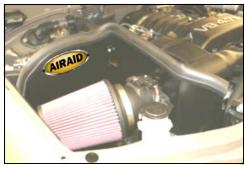
**10.** Install the Airaid Premium Filter (#1) on the MAF adapter. Next install the weather strip (#9) on the CAD as shown. Start at the front, next to the radiator, and work your way
