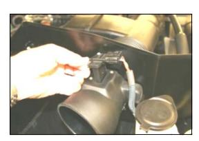
**8.** Re-route MAF wire harness under the intake tube, and around the front of the airbox. Install MAF sensor into the MAF adapter, using two supplied button head screws (#20). **DO NOT USE FACTORY SCREWS!**
