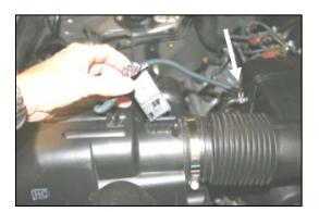
1. Disconnect negative battery cable. Remove 2 screws and remove and set aside the Mass Air Flow sensor from the factory airbox. Unclip wire harness from intake tube.
