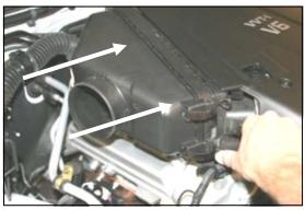
**9.** Re-install the factory airbox cover, and re-latch both clips.
