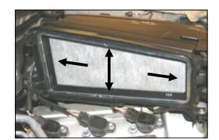
**7.** Re-install the gasket assembly back into the factory airbox as shown. Do not tamper with the factory hydrocarbon filter, as this will void the vehicle manufacturer's warranty, and street legal status in the state of California.
