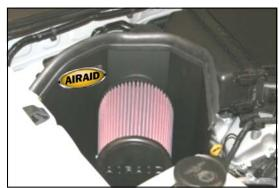
**15.** Install the Airaid Premium Filter (#1) on the **CAD** tube and tighten the clamp. Next install the weather strip (#7) on top of the **CAD** as shown. For an easier install, start at the fender side of the **CAD** and work your way towards the radiator.
