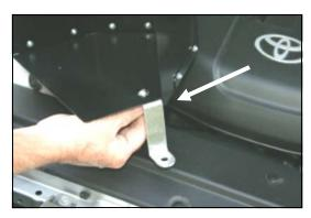
**12.** Install the bracket (#17) on the front of the **CAD** using the 1/4-20 button head bolt (#13), 1/4" flat washer (#14), and 1/4" serrated nut (#15), as shown. Just snug the bolt for now, there will be some adjustment needed once the **CAD** has been installed.
