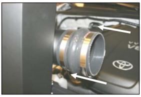
**11.** Install the urethane hump hose (#4), and two #64 hose clamps (#8) on the tube of the **CAD** as close to the panel as possible. Leave the hose clamps loose for now.
