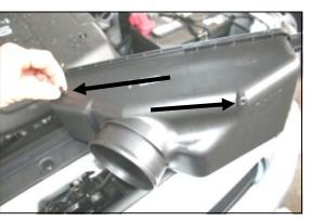
**8.** Install the two rubber washers (#19) onto the two plastic plugs (#18) that are provided in the hardware kit, and insert them into the two weep holes in the factory air cleaner cover removed in step #4, as shown
