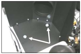
**13.** Install the **CAD** into the vehicle by aligning the hump hose with the tube on the factory airbox, and then aligning the two holes in the bottom of the **CAD**, and the bracket, with the three mounting holes on the inner fender. Install the three supplied 8mm bolts (#12) and washers (#15).
