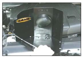
**10.** Assemble the Cool Air Dam panels (#2), and (#3) using the six supplied screws (#9), washers (#10), and nuts (#11.). Apply the Airaid Foil Decal onto the Panel as shown
