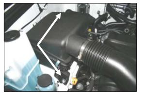
5. Using a 10mm socket, loosen the two bolts that anchor the factory airbox to the inner fenderwell. One is on the front of the airbox, and the other is on the rear. Pull the factory intake tube away from the throttle body and remove the corr
