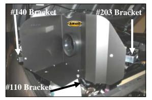
7. Assemble the Cool Air Dam panels (#3 & #4) as shown using four 6-32 screws (#9), washers (#10), and keps nuts (#11). Install the filter adapter (#5) using three 1/4" button head bolts (#13) and washers (#14). Install the 3 brackets (#24), (#25), and (#26) as shown using three 1/4" bolts (#13), washers (#14), and nuts (#15). Just snug the bolts for now, they will be adjusted later.Apply the Airaid Foil Decal onto the Panel as shown.
