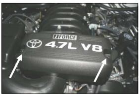
Disconnect the negative battery cable. 1. Using a 10mm socket, remove two nuts and the engine beauty cover. Set them to the side for now, they will be reinstalled in step #14.
