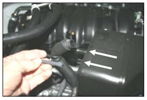
4. Disconnect the breather hose from the back of the factory intake tube and the valve cover. Disconnect the 1/8" vacuum hose from the back of the factory intake tube and the vacuum connection on the engine. These hoses will be replaced
