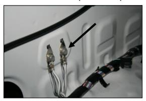
6. Using a 10mm socket, remove the rear ground anchor bolt on the passenger side inner fenderwell. Save the bolt, it will be reused in step #8.
