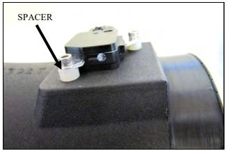
**8.** Transfer the Mass Air Flow sensor from the factory airbox, into the Airaid Intake tube and secure using the two #8 Spacers and 8-32 Socket Head screws . **Do not use the factory screws.**
