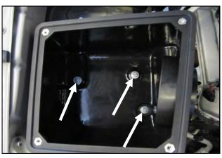
7. Mount the Cold Air Box onto the CAB Mounts using the three 8mm Bolts and 5/16 Flat Washers.
