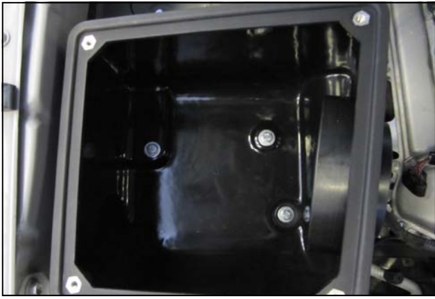
35. Mount the Cold Air Box onto the CAB Mounts using the three 8mm Bolts (#14) and 5/16 Flat Washers (#16).
