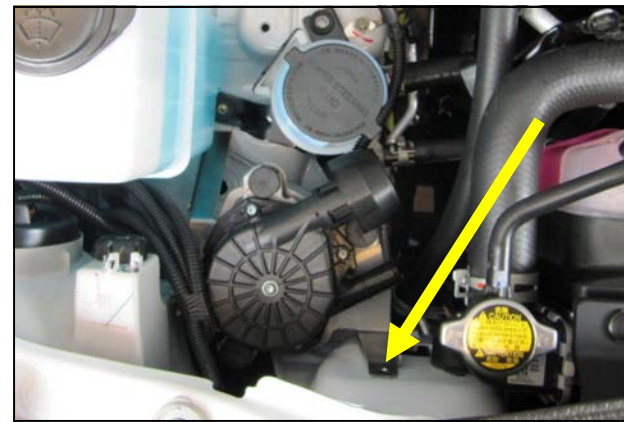
30. Reinstall the air pump assembly underneath the power steering reservoir bracket in the number 2 and 3 bolt holes from step 29. Finish the install by bolting the third Bracket tab to the vehicle using the 1/4-20 Button Head Bolt (#18), 1/4" Flat Washer (#19), and 1/4-20 Flange Nut (#20).
