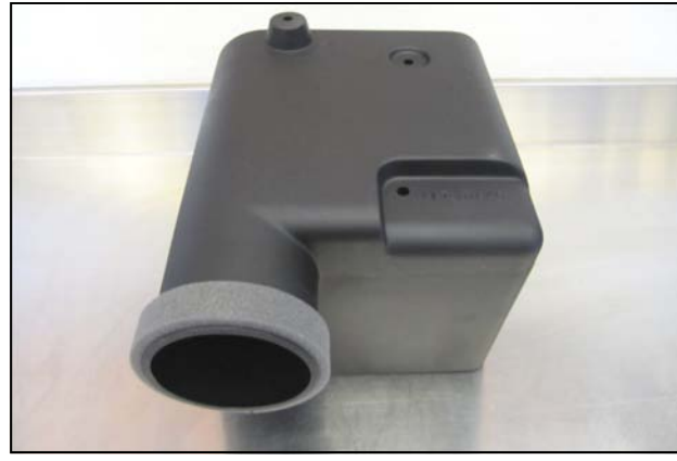
33. Apply the self adhesive, Foam Weatherstrip (#11) onto the air inlet on the Cold Air Box (#3).
