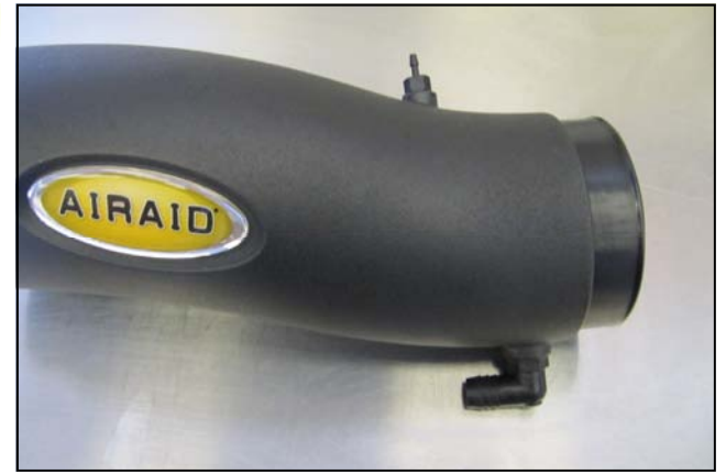
37. Install the 1/8" and 3/8" barbed fittings (#s 13 and 14) into the Airaid Intake Tube. Apply the Airaid Bubble Decal onto the Intake Tube as shown.
