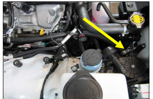
31. Connect the 3/4" hose from step 17 to the air pump outlet and re use an OEM spring clamp to secure it.
