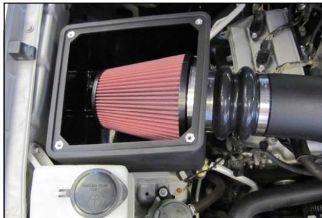
41. Install the Airaid Premium Filter onto the Filter Adapter inside of the airbox and tighten the clamp.
