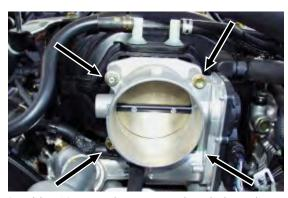
4. With a 10mm socket, remove three bolts and one nut from the throttle body. Slide the throttle body away from the intake manifold, and remove the remaining stud.
