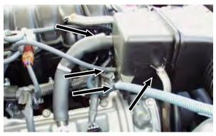
3. Disconnect the breather hose, and two vacuum lines from the back of the intake tube. Remove the clip from the back of the intake tube that holds the wiring harness, these will all be re-connected later. Remove the intake tube from the vehicle.
