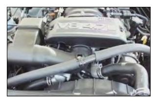
6. Re-install the intake tube and tighten the hose clamps. Re-connect the vacuum lines, wiring harness clip, and breather hose. Re-install the bolt thru the clamp on the air conditioning hose into the intake tube. Re-install the beauty cover and nuts. **Re-connect the negative battery cable!**
