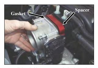
5. Install the Airaid spacer next to the intake manifold, and the fiber gasket next to the throttle body. Insert the four provided 6mm bolts, and washers, and tighten in a cross pattern, to the vehicle manufacture's specifications.
