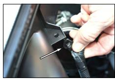
2. Carefully remove the lid, turn it over, and pinch the two tabs together to remove the plastic wiring harness holder from the lid (If equipped). Now remove the lid from the vehicle and set it aside, it will be reinstalled later.
