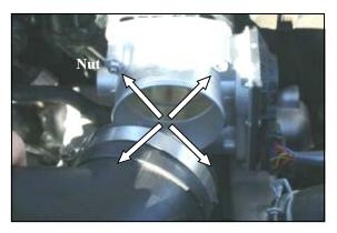
**3.** Using a 10mm socket, remove three factory bolts, and one nut. Pull the throttle body towards the radiator until it clears the stud, and then move it aside.
