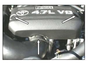
**6.** Re-install the intake tube and engine beauty cover. **Reconnect the negative battery cable!**
