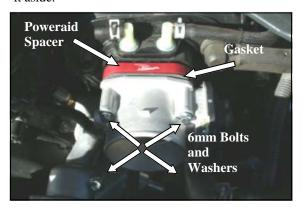
**5.** Position the Poweraid Spacer (#1) and gasket (#2) between the throttle body and intake manifold. Insert four 6mm x 65mm hex bolts (#3), and 6mm flat washers (#4) thru the throttle body, gasket, Poweraid Spacer, and into the intake manifold. Using a 10mm socket, tighten all four throttle body bolts evenly, to the manufacturers specifications. **Do Not Over Tighten The Bolts!**
