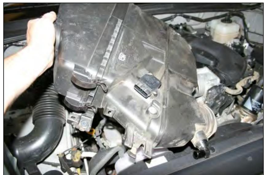
**4.** Remove the complete resonator/airbox assembly from the vehicle.
