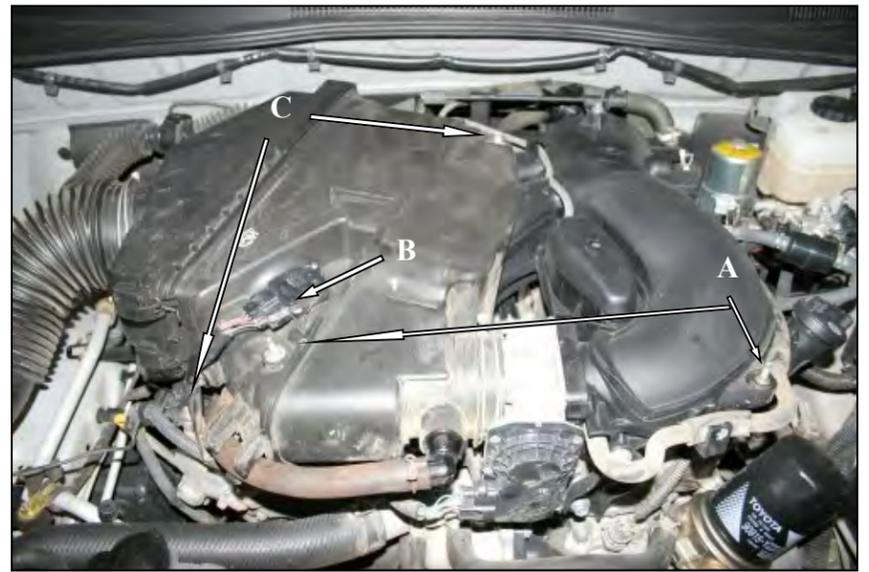
**2. A.)** Using a 4mm socket, remove the two studs that secure the beauty cover to the engine.
