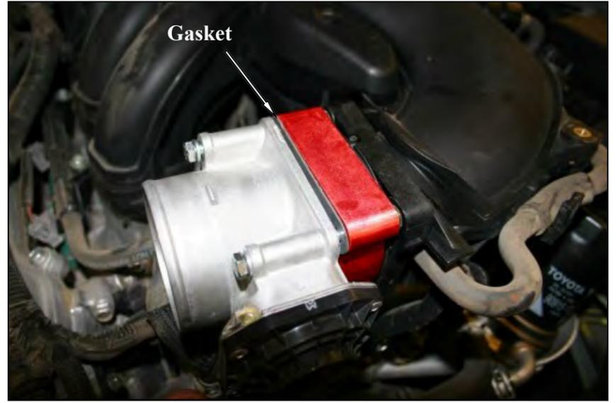
6. Slide the Airaid Spacer (#1) and gasket (#2) between the intake manifold and the throttle body. Make sure the "Flow" arrow on the spacer is pointing towards the intake manifold, and the gasket is next to the throttle body. Install the 4 supplied 6mm x 75mm bolts (#3) and flat washers (#4) thru the throttle body, gasket, spacer, into the intake manifold and tighten evenly to the vehicle manufacturer's specifications.
