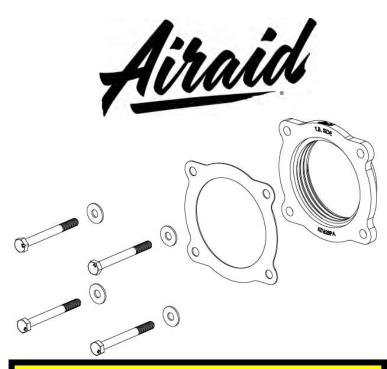
**Installation Instructions** Part Number 510-628 **AIRAID Spacer For** 2010-2014 Toyota FJ Cruiser 2010-2020 Toyota 4Runner 4.0LV-6
