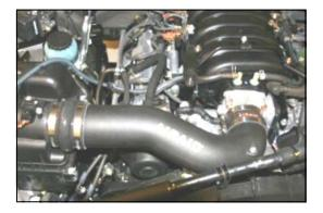
9. Install the MIT into the hump hose first, and then into the reducing coupler. Adjust the MIT snugly against the throttle body, and tighten the 4 hose clamps. Next install the  $1/4 - 20 \times 1/2$ " button head bolt (#10) and 1/4" flat washer (#11) thru the Adel clamp and into the MIT to hold the air conditioning hose.
