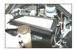
6. Remove the factory air filter, and install the iraid Premium Filter (#1). Reinstall the facto
