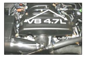
1. Disconnect negative battery cable. A) Using a 10mm socket, remove the two 10mm nuts, and remove the beauty cover. (Save for reuse). B) Remove the bolt thru the Adel clamp that holds the air conditioning hose.
