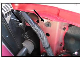
**14.** Place Well Nut into 3/8" hole in core support.
