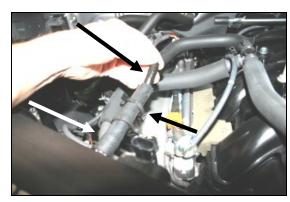
**12.** Install the 1/2" breather hose (#23) onto the nipple on the Airaid tube. Slide the 1/2" barbed coupler (#21) into the installed breather hose, and secure both ends with the supplied speed clamps (#22)
