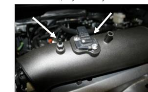
9. Re-install the MAF sensor into the Airaid intake tube (#2) as shown using the supplied 8-32x3/8" button head screws (#12). **Do Not Use The Factory Screws!** Next install the 1/8NPTx3/16" barbed fitting (#20) into the Airaid tube.
