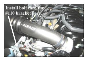
11. Install the Airaid intake tube into the hump hose first, and then into the reducing coupler. Center the tube between the throttlebody, and the CAD, adjust for fit, and then tighten the four hose clamps. Install one 6mmx12mm bolt (#16) and washer (#14) thru the bracket into the captured nut in the fender well.
