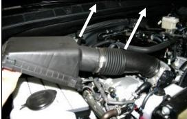
box lid to the base and remove the intake tube and lid from the vehicle. Remove the factory air filter
