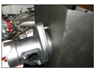
7. Using two supplied ½-20 bolts and washers, mount the Airaid filter adapter to the Airaid Cool Air Dam.
