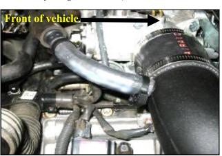
14. Using the supplied 5/8" to ½" barbed connector and ½" x 4" breather hose, connect the factory hose located by the throttle body to the Airaid intake tube. Use two supplied #16 Speed clamps to secure the hose to the barbed ends.
