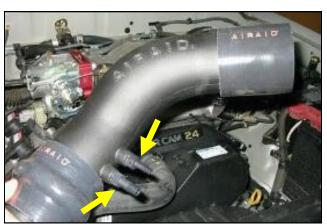
9. Install two supplied 1/4" NPT barbed fittings in Airaid intake tube. (Note: Install 3/8" fitting in the forward hole and the 1/4" fitting in the back hole) Slide hump hose and two #52 hose clamps on large end of intake tube and slide coupler with two #48 hose clamps on small end of tube. (Note: leave all hose clamps loose for final assembly)
