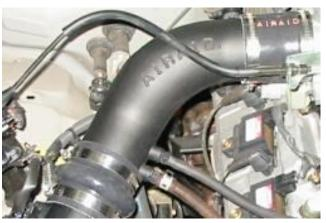
11. Connect the Airaid intake tube to the engine by sliding the coupler over the throttle body & adjust the intake tube to insure proper alignment from the throttle body to the air filter adapter. (Note: Leave a gap between the tube and the air filter adapter to allow for engine movement)
