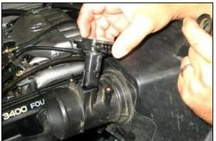
**5.** Loosen the two screws on the Mass Air Sensor and remove the sensor from the factory air box. <u>Retain sensor for later use.</u>
