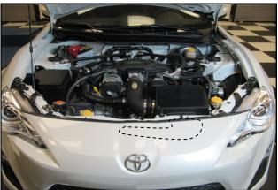
With help from an assistant. The inlet can be removed without removing the entire bumper cover. Simply remove all of the topside fasteners and pull back on the cover. Have an assistant remove the two 6mm bolts in the tube and remove.
