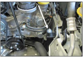
5. Install the CAB Mount (#16) into the airbox bracket on the inner fender. Hand tight is sufficient.
