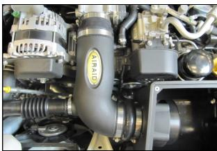
**12.** Install the Intake Tube and tighten all of the clamps. Connect the crank case breather to the Barbed Fitting and secure it using the OEM spring clamp. Insert the resonator into the Intake Tube and tighten the clamp.
