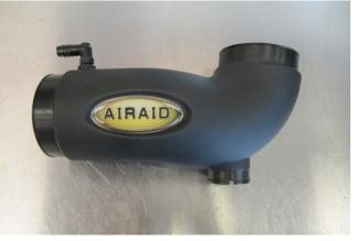
11. Install the Barbed Fitting into the Intake Tube and apply the Airaid Decal, as shown.
