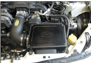
**15.** Install the Air Box Lid using the 10-24 Button Head Screws and the #10 Washers.
