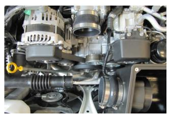
**10.** Place the Hump Hose and two #52 Clamps onto the Filter Adapter and the Reducer with one #52 and one #44 Clamp on the throttle body. Leave the clamps loose for now.
