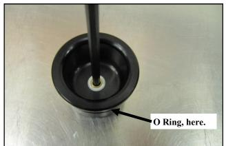
Apply a thread sealer to the threads of the Brass plug and insert it into the Sound tube plug. Slide the O Ring onto the plug and into the groove. Install the Plug Assembly into the Intake tube port and secure using the #24 Clamp. It should be noted that the Aluminum is designed to accept many 1/16 NPT N2O foggers
