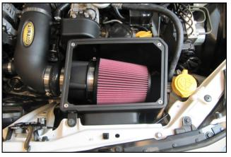
**13.** Install the Airaid Premium Filter onto the Filter Adapter.
