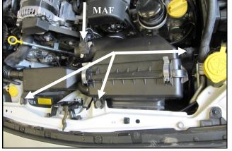
2. Disconnect the Mass Air Flow sensor, or MAF, in the airbox. Remove the three 6mm bolts securing the airbox assembly and remove it from the vehicle.
