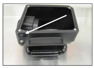
**6.** Mount the Airbox Bracket as shown, using one 1/4-20 Button Head Screw and a 1/4" Flat Washer. Transfer one factory airbox mounting grommet and steel sleeve from step 3 into the Airbox Bracket.
