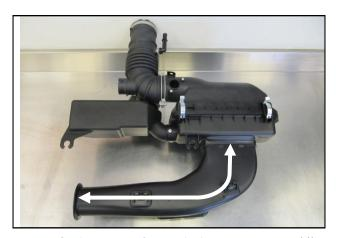
**Install Option Two: OEM air inlet removal.** While not necessary, maximum power is achieved by removing the OEM inlet from the vehicle.
